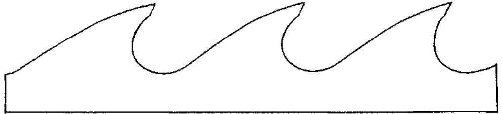
Figure 12. Pattern of saw teeth used with a 14-inch 13-gauge band headsaw.
