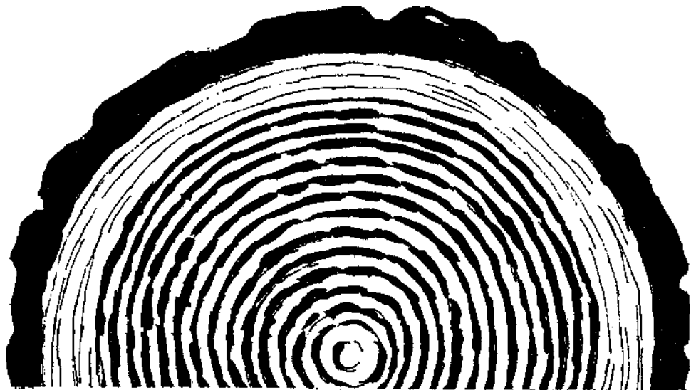
Figure 17. End section of a log, showing pith, truewood, sapwood and bark.
